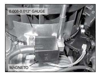
Figure 34. Setting Ignition Magneto (Armature) Air Gap
